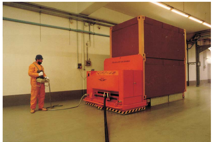
Top and bottom: Up to 40t moves this remote-controlled air-cushion transporter, which is special designed for the use in nuclear plants (BLG-Gorleben).
