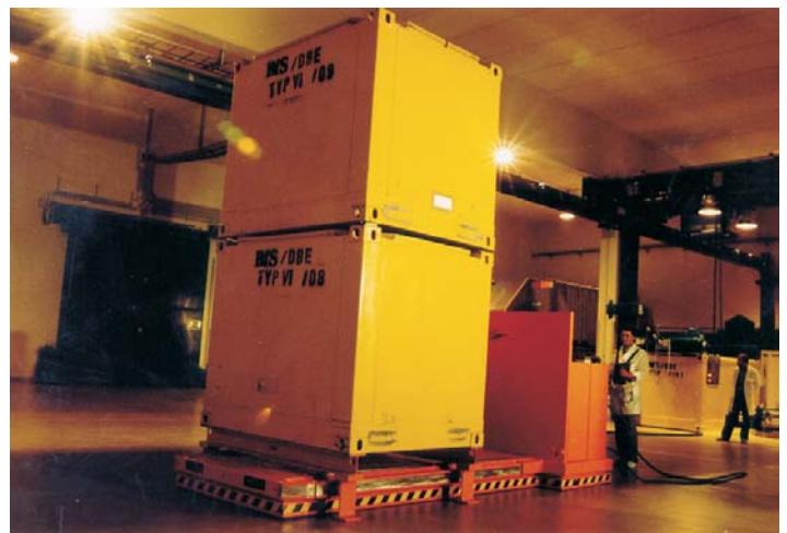
Top and bottom: Up to 40t moves this remote-controlled air-cushion transporter, which is special designed for the use in nuclear plants (BLG-Gorleben).
