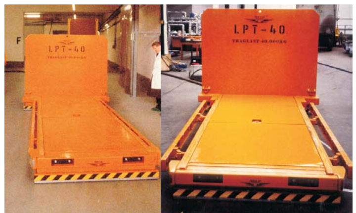
At the right picture you see the fixture for automatic centering below the load.
