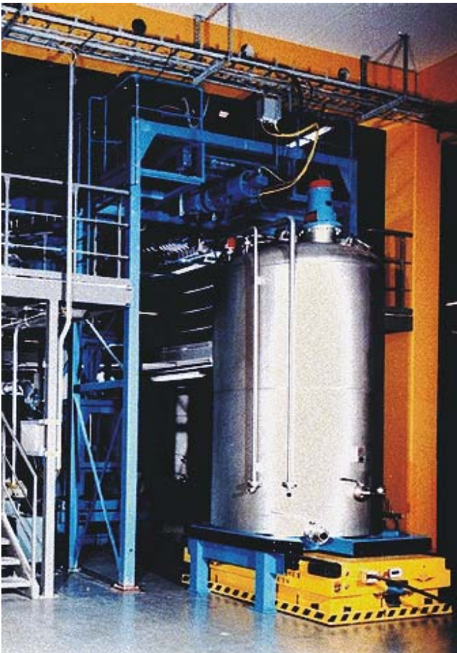
Pic. 1: A paint-vessel is moved into the dosing station.
