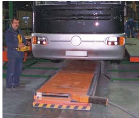
1: Remote controlled air-cushion transporter for buses
