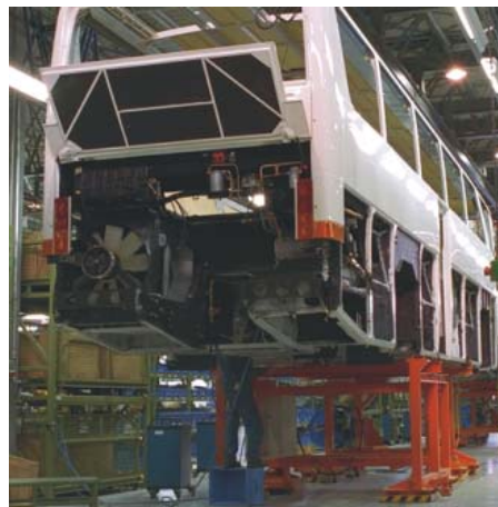
2: Air-cushion transporters for underfloor works
