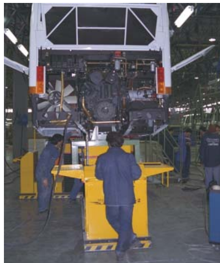
3: Air-cushion-device for the assembly of engines
