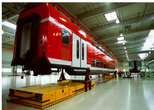
Fig. 4: Tape guided AGV with air-cushion gear for the transport of railcars (Duo operating mode)
