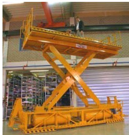
Fig. 2: Autonomous working platform with an air-cushion gear, for the flexible use.
